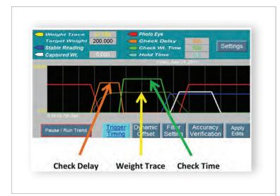
Built-in VISUALIZATION TOOLS eliminate the trial and error of product set-up, enabling operators to capture the entire checkweighing process and display results on the machine's high-resolution HMI screen. Operators can quickly and easily determine the perfect set of parameters to maximum weight capture time and optimize for repeatability and accuracy.
